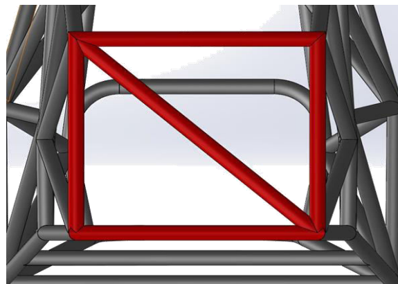
Fig -9: Front bulkhead design
