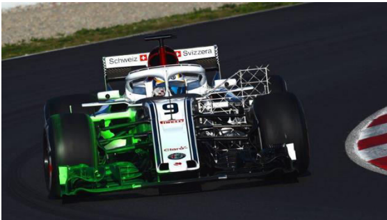
Fig 15: F1 C37 car testing wind flow with the help of fluid
